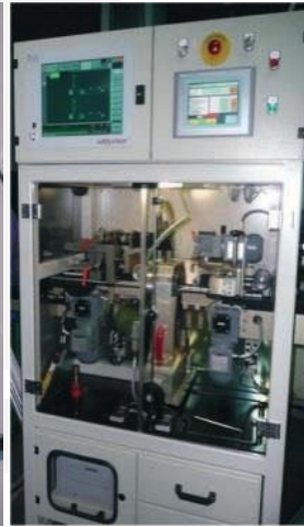
Crack detection EDDY currents
