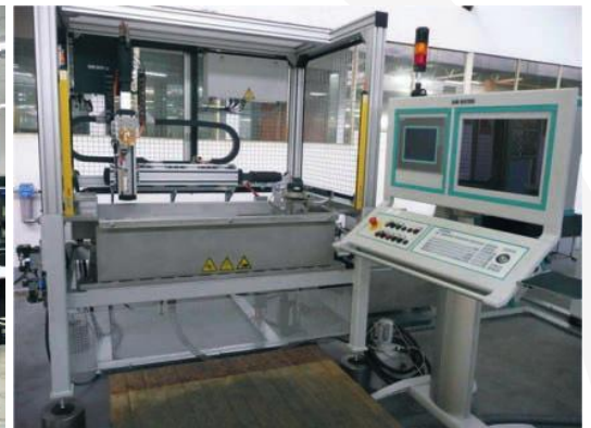
Crack detection - Ultrasonic
